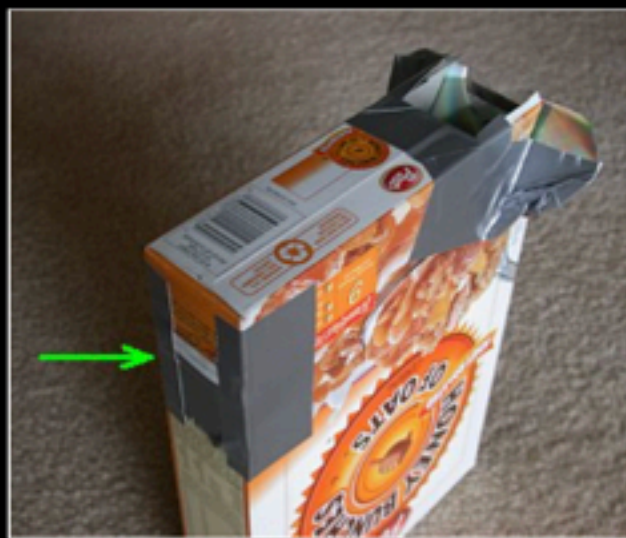
my cereal box spectroscope (arrow: the slit)
